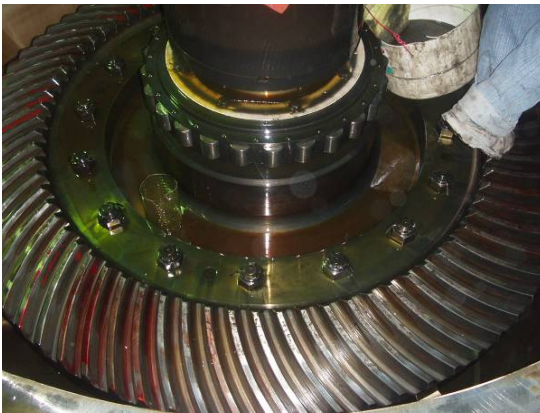
Gear replacement at Raw Mill
