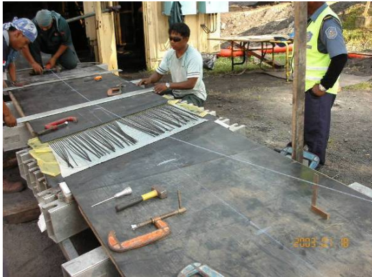
Steel Cord joint at Kapar Power Plant
